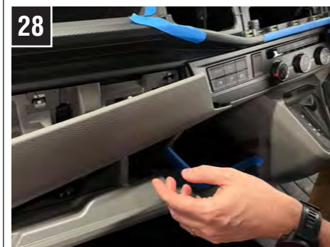
Remove the panel above the glovebox using a panel removal tool to release the clips highlighted in step 29.
