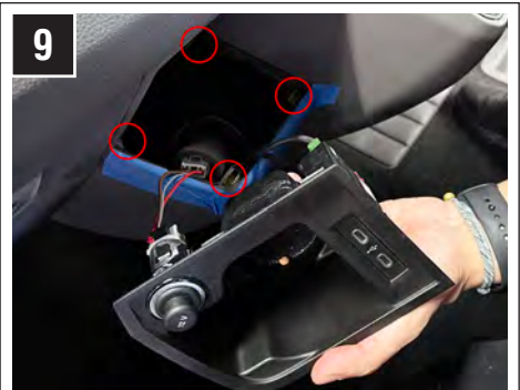
9 The highlighted clips secure the panel. Once released carefully lift from the dash ready to disconnect the OEM connectors. (See step 10)
