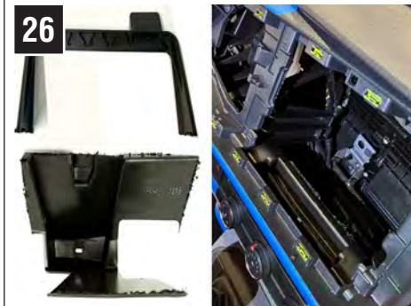
On the left are the cut panels from dashboard. On the right shows the dashboard once cut and ready to install the aftermarket stereo. Dispose of any recyclable components in accordance with local regulations.
